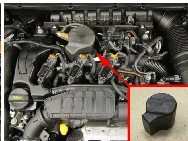
Hose routing. Adapt & mount pump cover.
