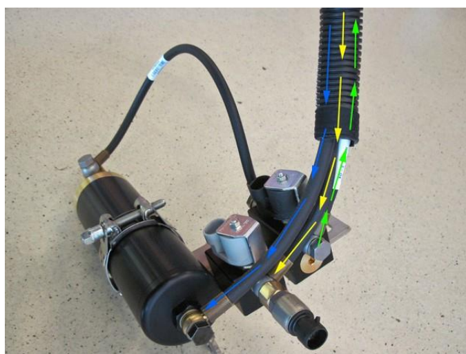
Mount fuel units and boost pump on bracket. Mount hoses.
