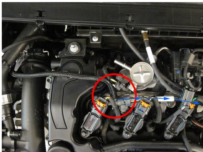
Connect supply hose to original fuel line (to boost pump).
