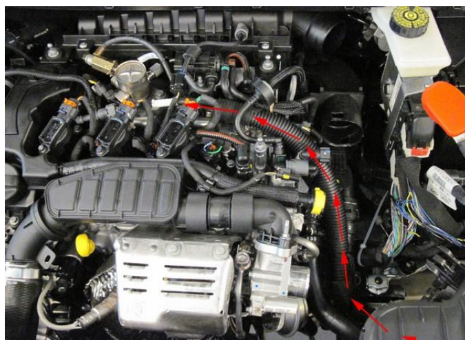
Hose routing. Adapt & mount pump cover.
