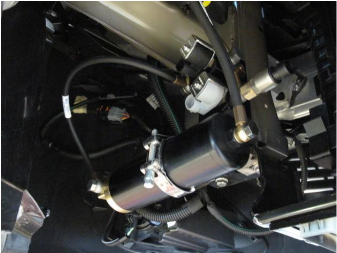
Mount shim around bolt. Mount fuel Unit.
