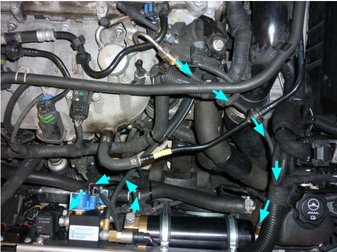
Fuel line to the boost pump and boost pump to the FSU.
