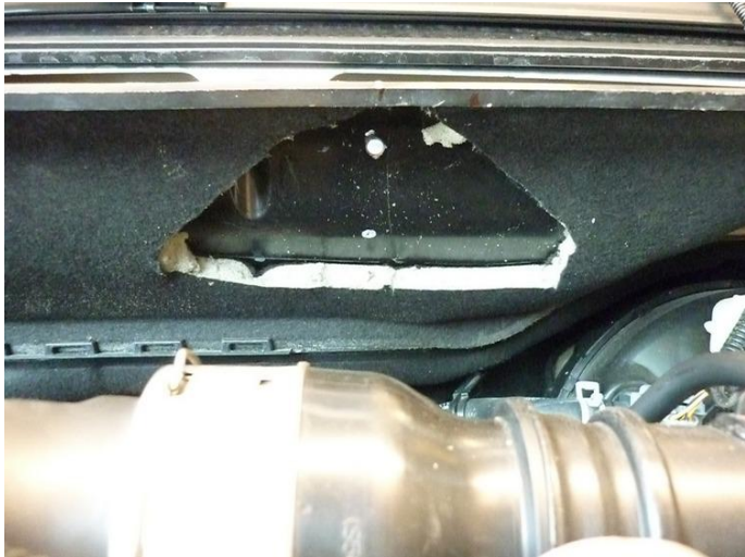
Mark, remove foam, mark holes, drill Ø7mm
