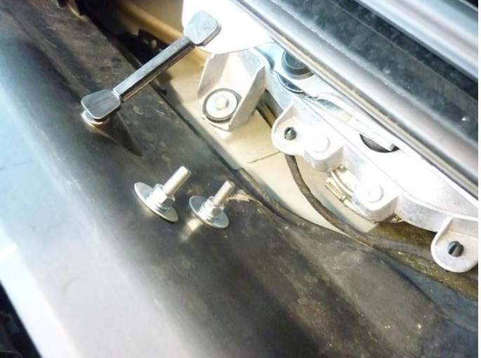
Mark, remove foam, mark holes, drill Ø7mm
