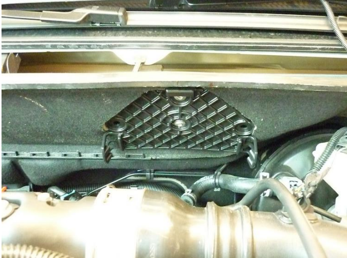
Mark, remove foam, mark holes, drill Ø7mm
