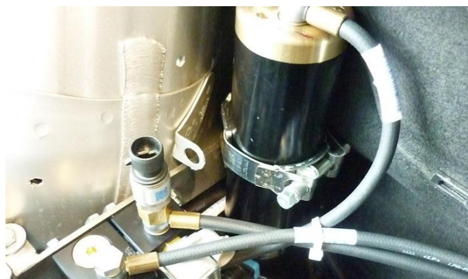
Hose with split tube and spacer clip on AC pipe
