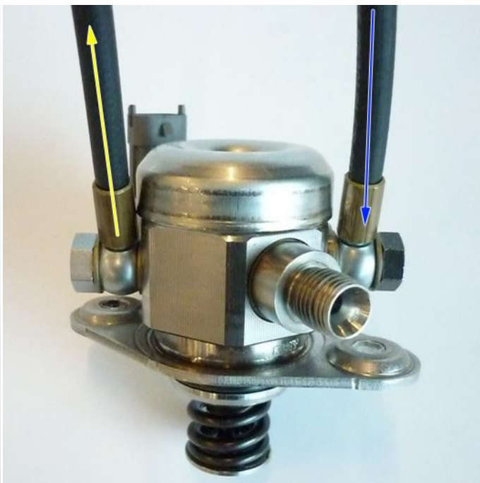
Adapted pump / pump with return and supply hoses; inlet: filtered banjo
