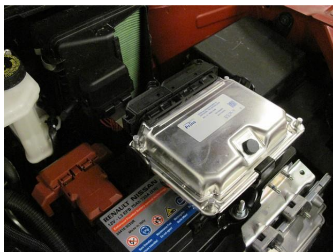
Mount the plastic AFC clip, AFC and fuse-relay box.
