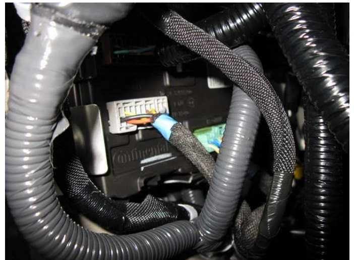
Loosen cover for easy access to the body control module for connecting the wake-up.
