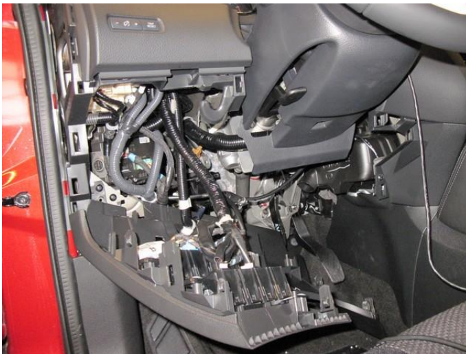
Loosen cover for easy access to the body control module for connecting the wake-up.
