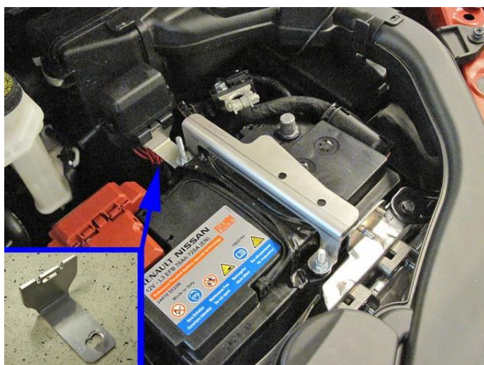
Mount the AFC & fuse-relay bracket to the original threaded rods from the battery clamp.
