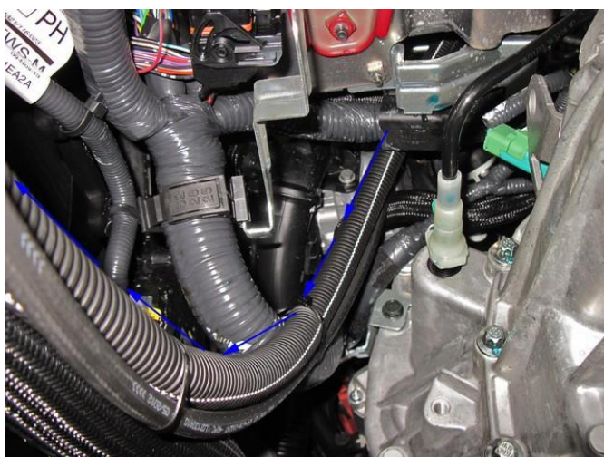
Mount hoses from high pressure pump to FSU & FRU.
