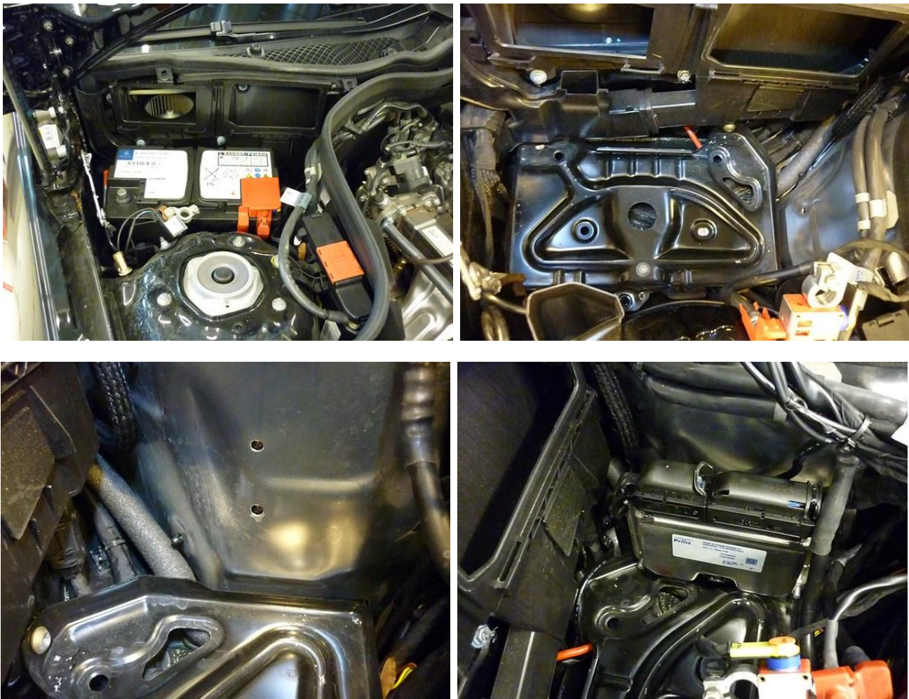
Drill 2x Ø8mm, install AFC-clip with 2 push clips
