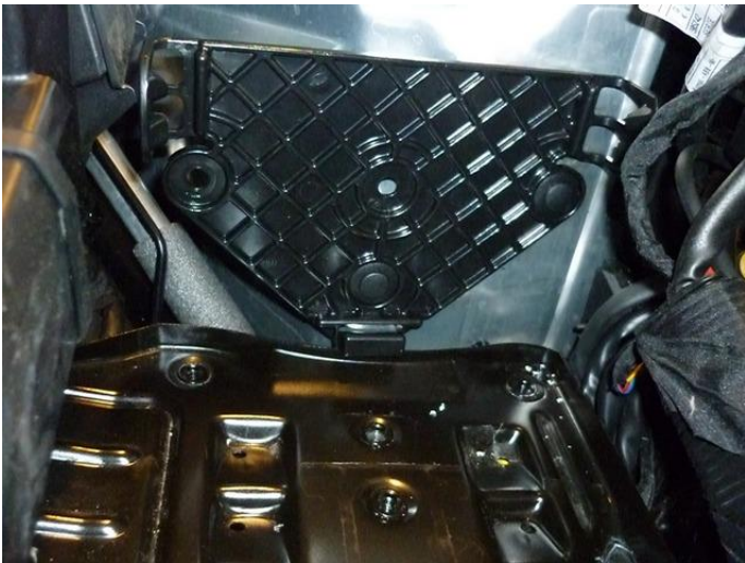
Drill 2x Ø8mm, install AFC-clip with 2 push clips
