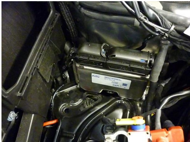
Drill 2x Ø8mm, install AFC-clip with 2 push clips
