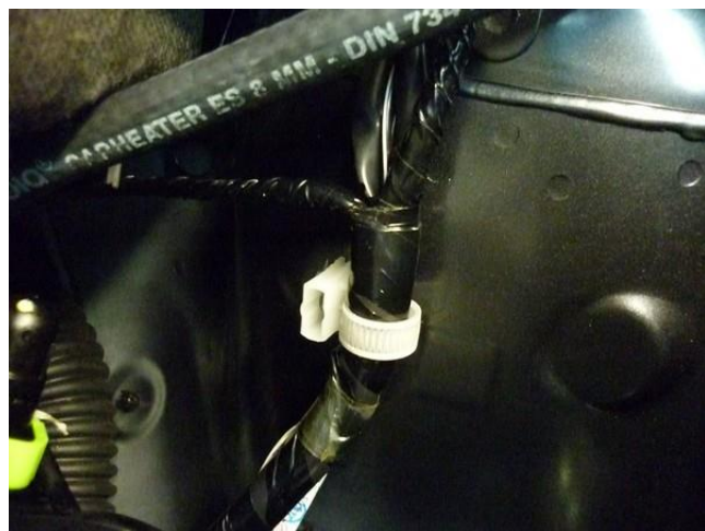
Replace white cable clamp, wiring loom moves to front
