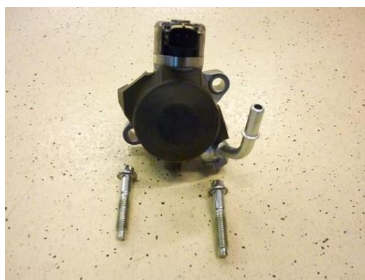
Remove high pressure petrol pump, not used anymore.
