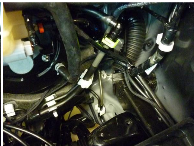
Replace white cable clamp, wiring loom moves to front
