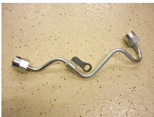
Remove/replace fuel line, reuse clamp.
