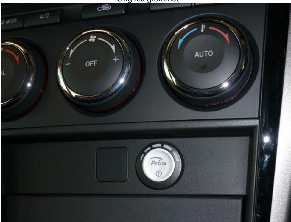
Drill Ø8,2 mm for the switch
