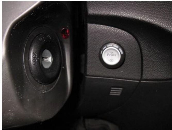
Mark & drill Ø8,3mm on the right side of the steering column. Mount fuel switch.
