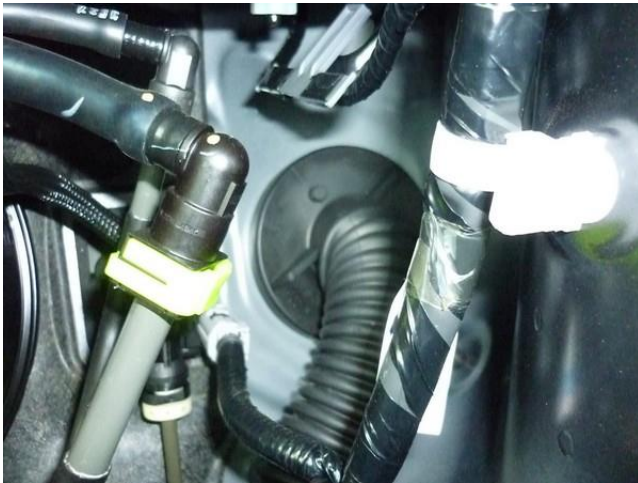
Grommet for putting through the Switch and CAN wiring ( before unit installing )
