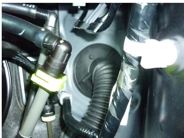
Grommet for putting through the Switch and CAN wiring ( prepare before unit installation )
