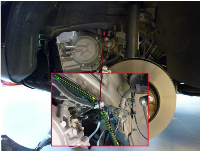
Install fuel lines for FSU and FRU
