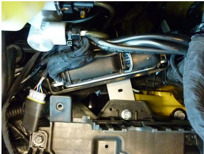
AFC mounted and ground point
