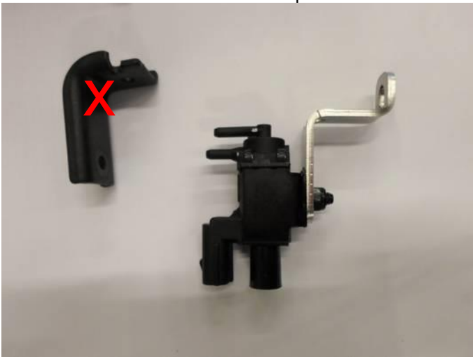
Remove original bracket place new bracket
