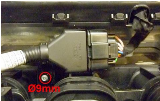
Drill up connector bracket
