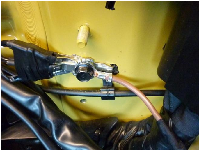
AFC mounted and ground point
