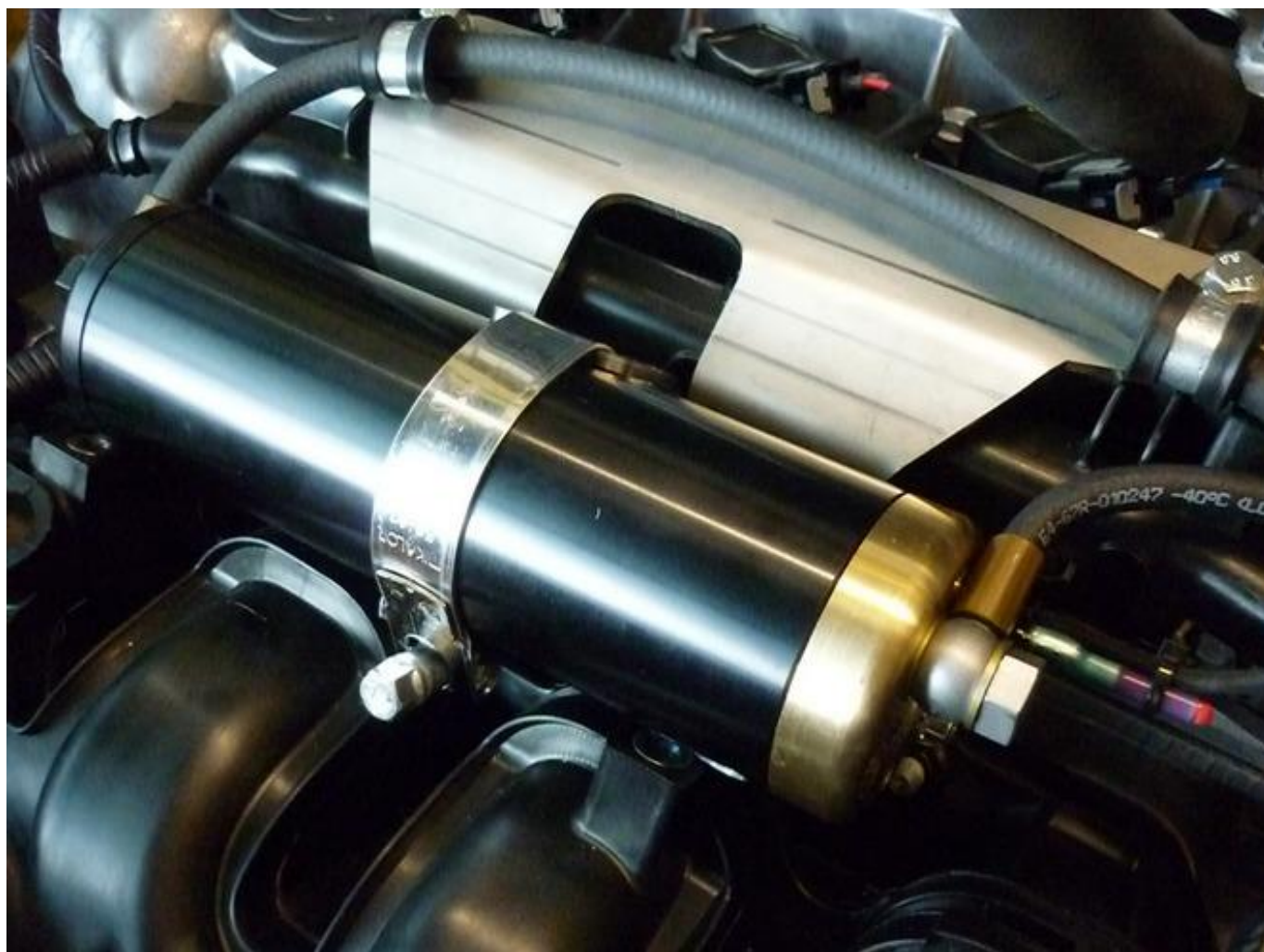
Boost pump clamp: 7Nm
