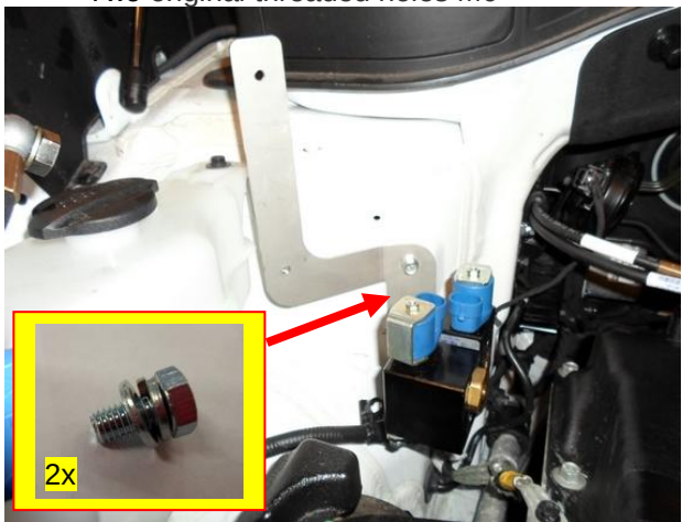
Two original threaded holes M6
