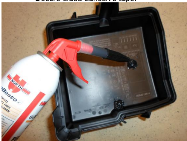
Seal the push pin rivets with silicone sealant.
