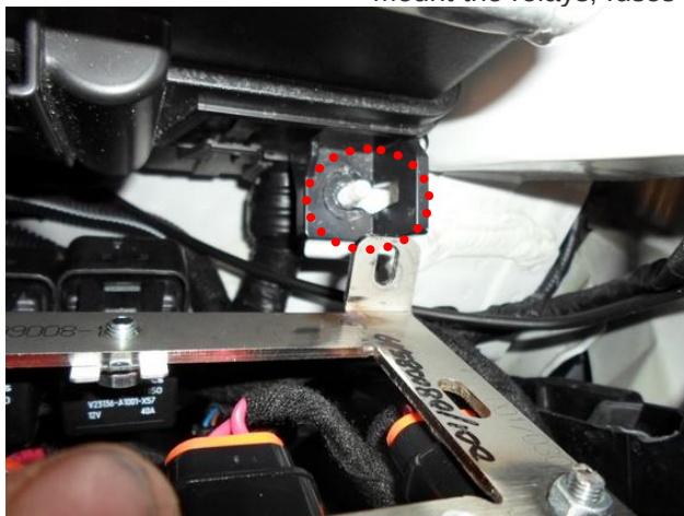
Mount the bracket under the fuse box. Use original M6 nut.
