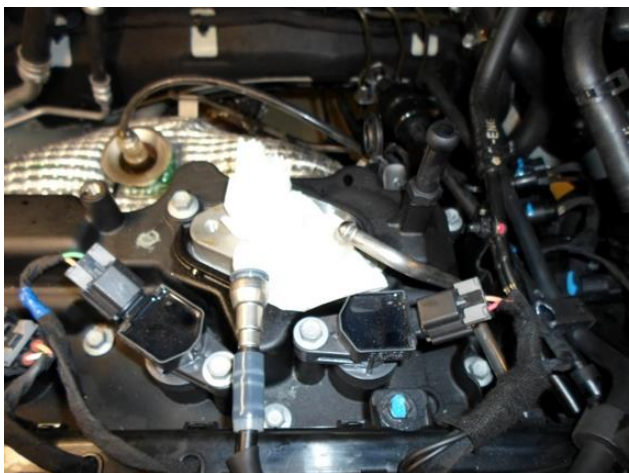
Cover pump housing until the adapted high pressure pump is mounted.
