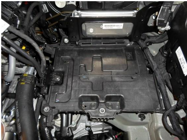
Install the battery mounting plate back.
