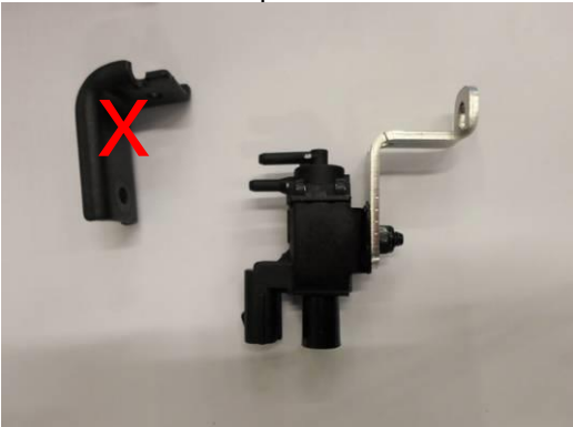
Remove original bracket place new bracket
