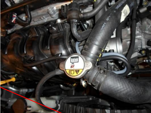
Install a new longer hose to the valve and cut 8cm off the original long hose
