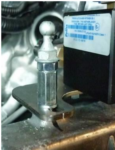
Original stud bolt with M6 nut
