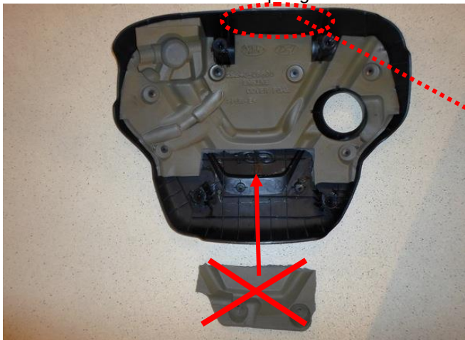
Adapt engine cover on the back side
