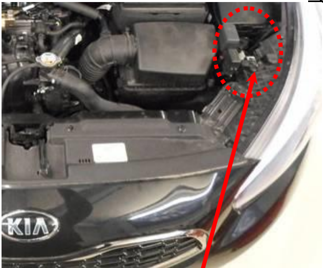
Fuse relay box and diagnose connector .
