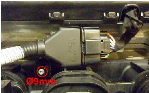
Drill up connector bracket
