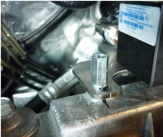
Spring washer and extended nut
