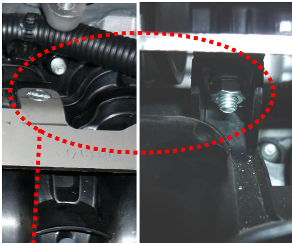
Bolt on the bracket with flush bolts M6 and nuts.
