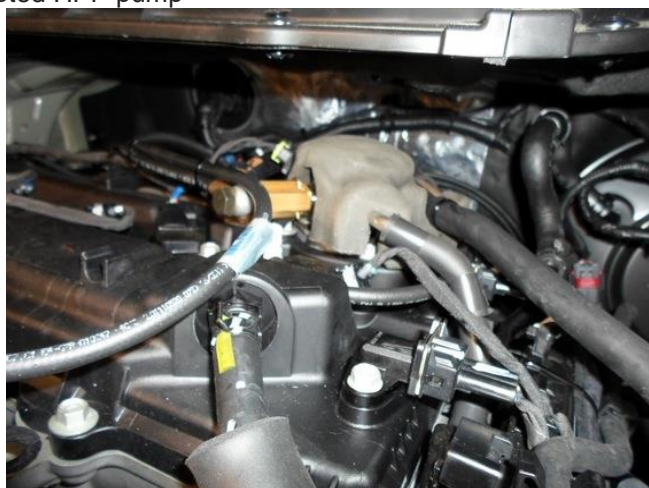
Install the adapted HPP pump
