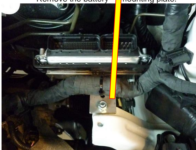
Remove the battery mounting plate.
