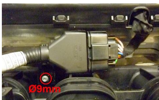
Drill up connector bracket
