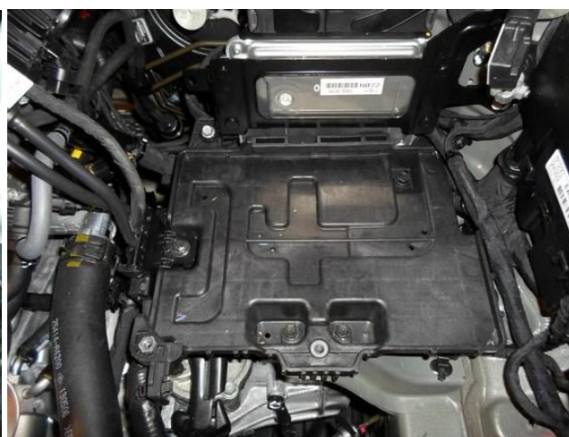
Install the battery mounting plate back.
