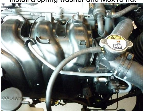
Install a new longer hose to the valve
