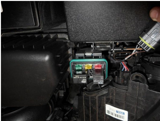
Fuse relay box and diagnose connector. Mounting point original M6 nut
