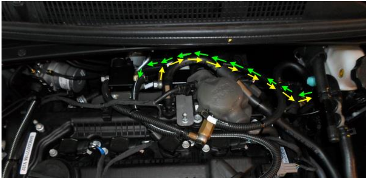
LPG TANK TO FSU AND FRU TO LPG TANK
