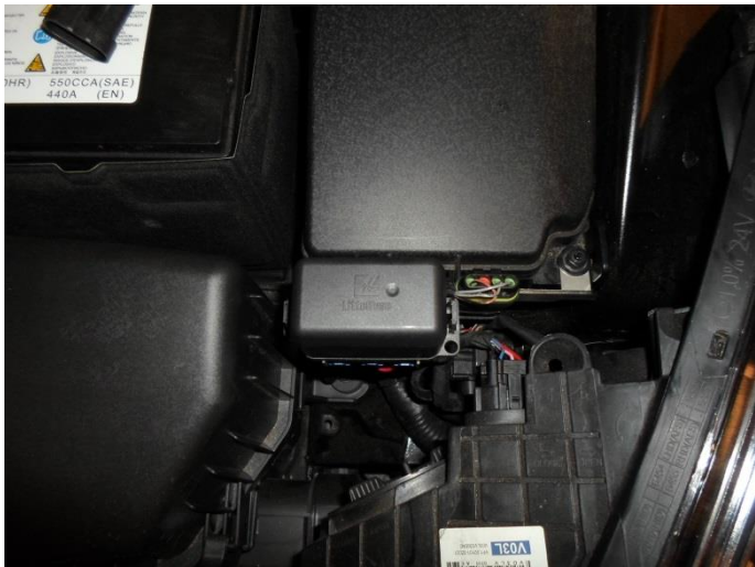
Fuse relay box and diagnose connector. Mounting point original M6 nut
