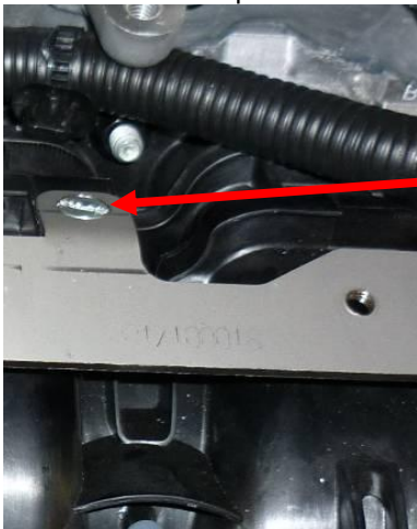
Bolt on the bracket with flush bolts M6 and nuts.
