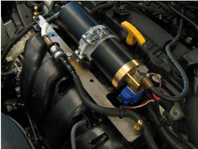
Bolt on the bracket with flush bolts M6 and nuts.
