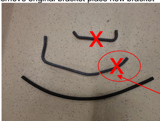
Install a new longer hose to the valve and cut the long hoses in 8cm
