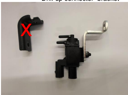
Remove original bracket place new bracket
