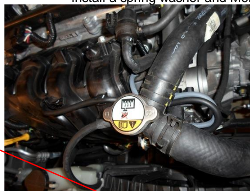
Install a new longer hose to the valve and cut the long hoses in 8cm
