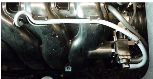
Install new longer hose to valve
