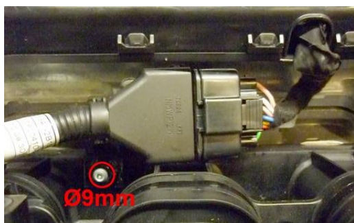
Drill up connector bracket
