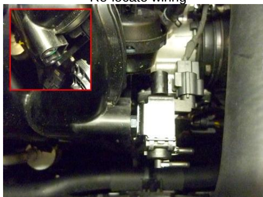
Install new longer hose to valve
