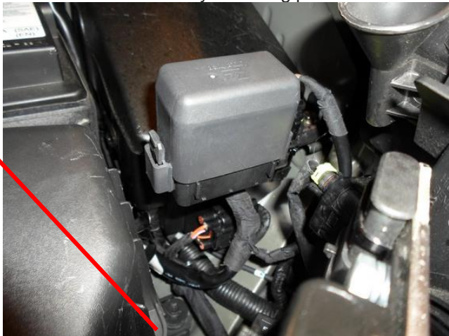
Mounting point original m6 nut
