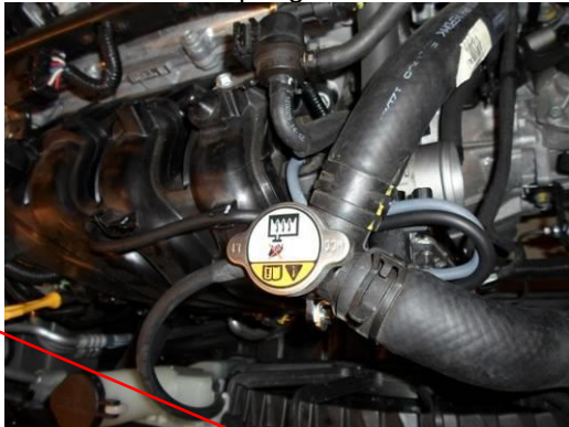
Install a new longer hose to the valve and cut off 8cm of the original long hose
