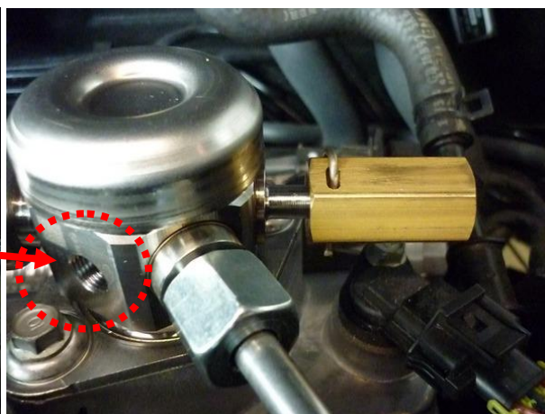
Replace for the adjusted high-pressure pump.
