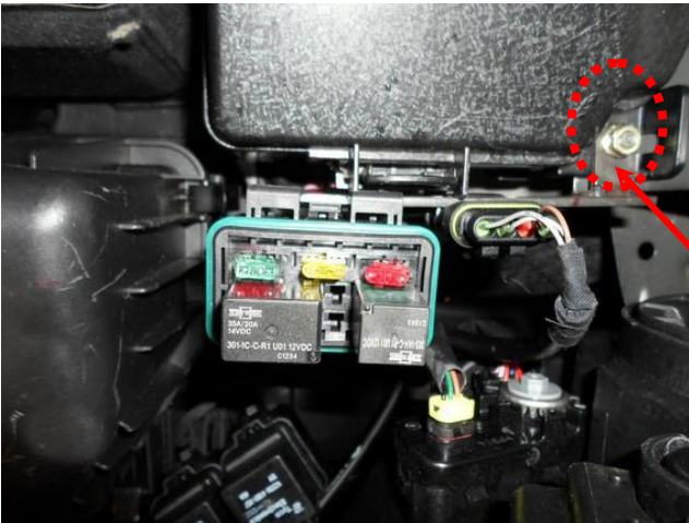
Fuse relay box and diagnose connector .
