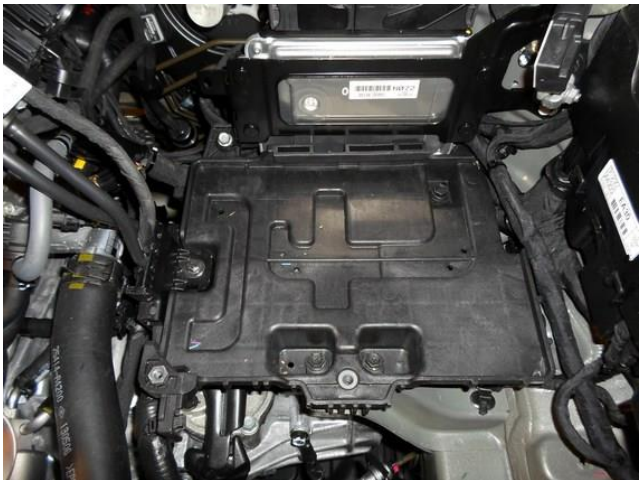
Install the battery mounting plate back.
