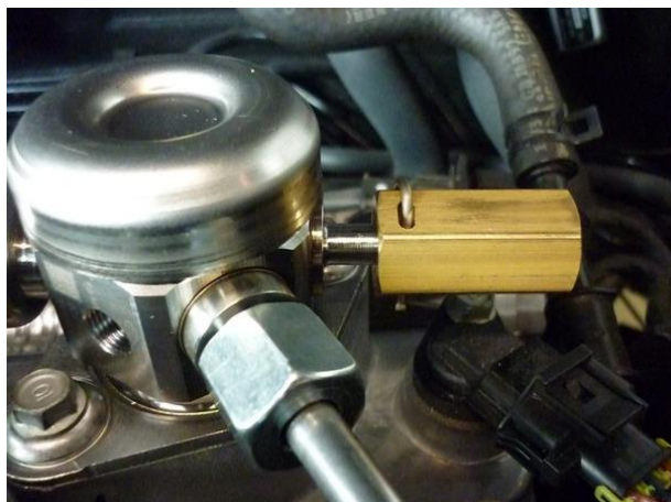
The adjusted high-pressure pump.
