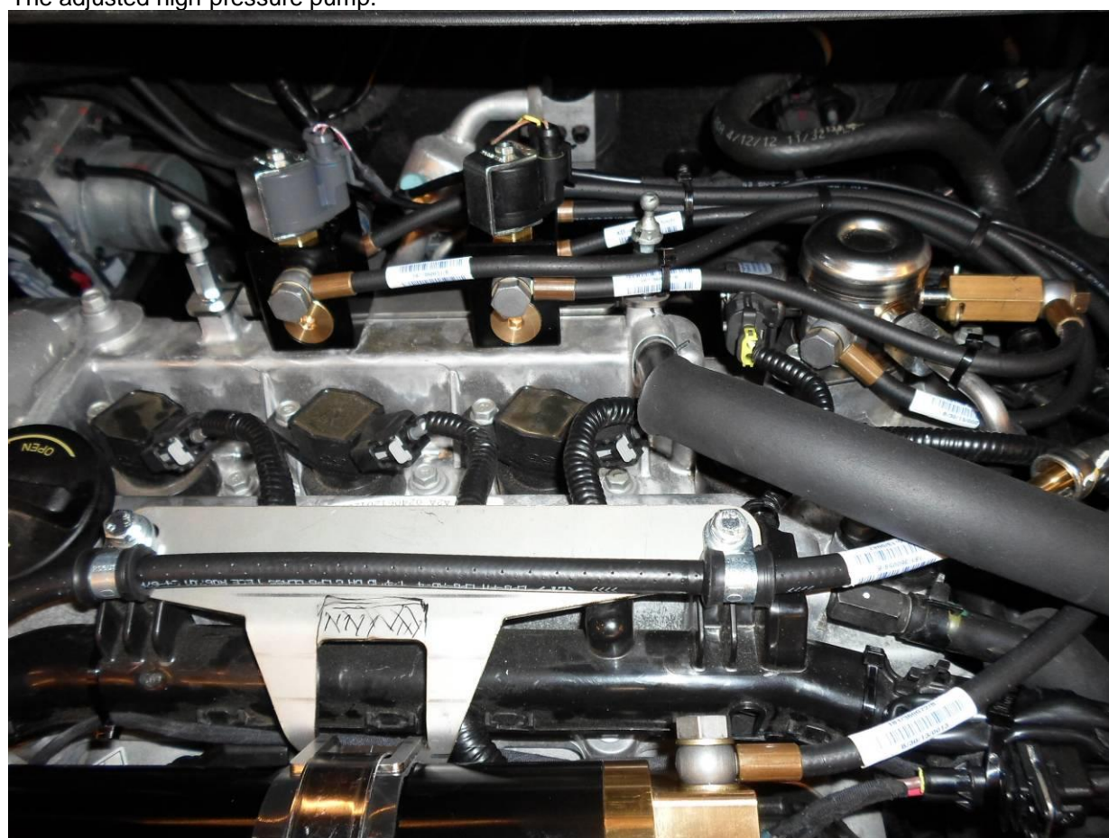
The adjusted high-pressure pump.
