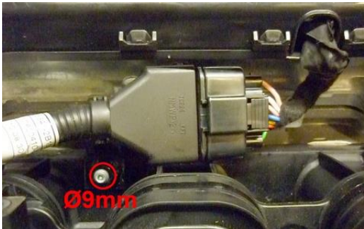
Drill up connector bracket
