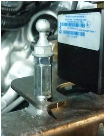
Original stud bolt with M6 nut
