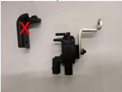
Remove original bracket place new bracket
