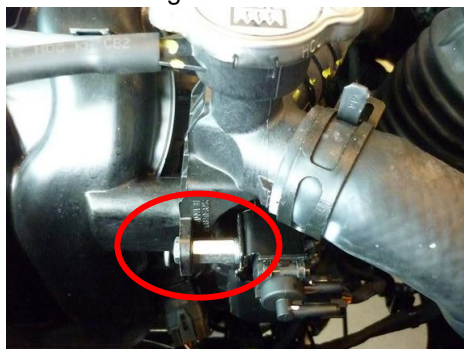
Install new longer hose to valve
