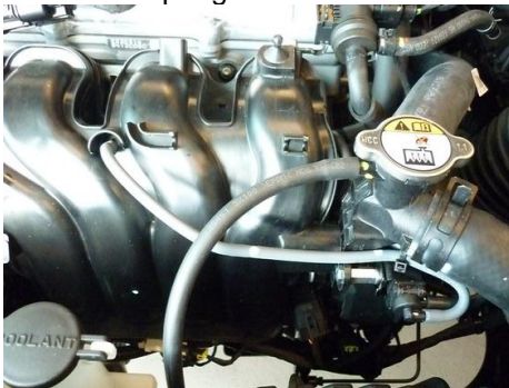
Install new longer hose to valve
