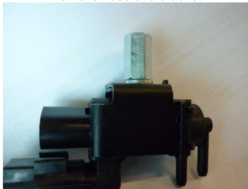
install a spring washer and M6x18 nut
