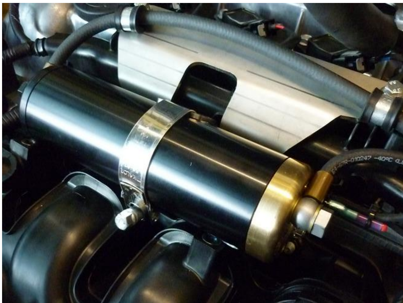
Boost pump clamp: 7Nm
