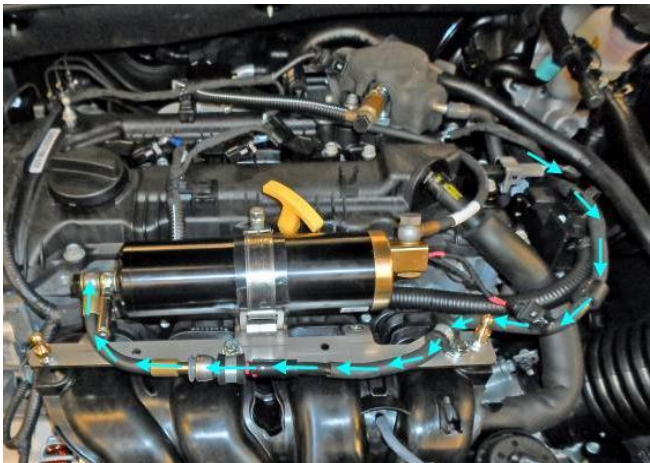
Original fuel line with extension line to boost pump
