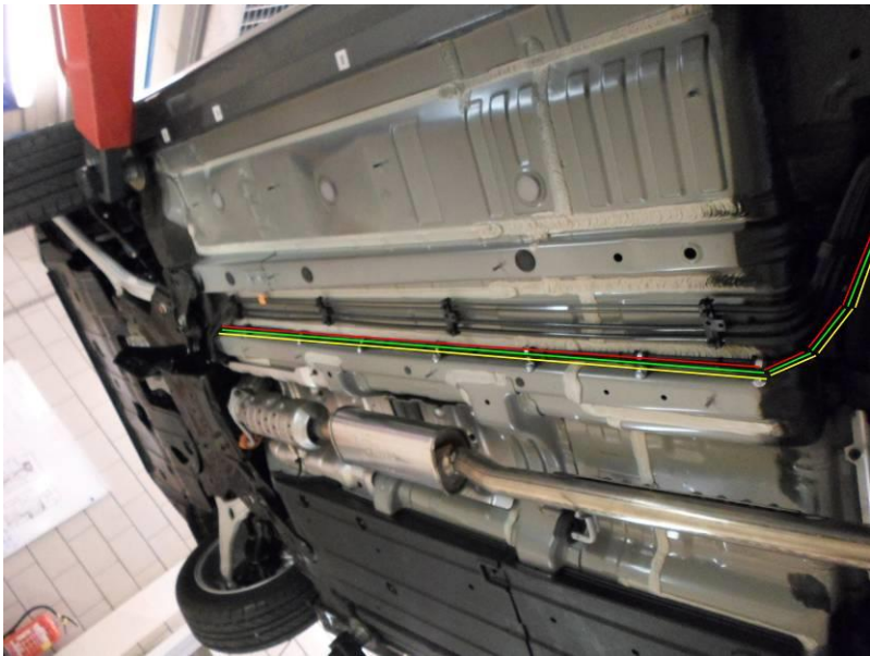
Mount 700mm protective tube around hoses from FSU&FRU to tank in the engine room.
