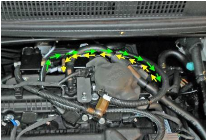
Mount 700mm protective tube around hoses from FSU&FRU to tank in the engine room.
