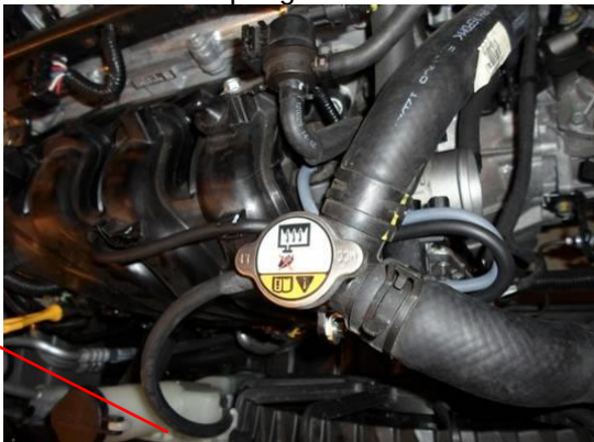
Install a new longer hose to the valve and short hose with 8 cm.
