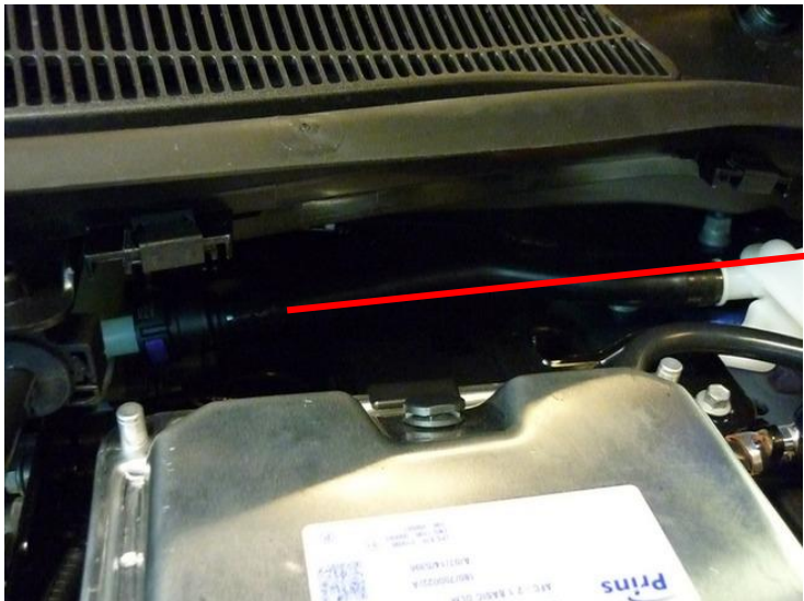
Original Grommet for switch and Can wiring, left side, above clutch pedal.
