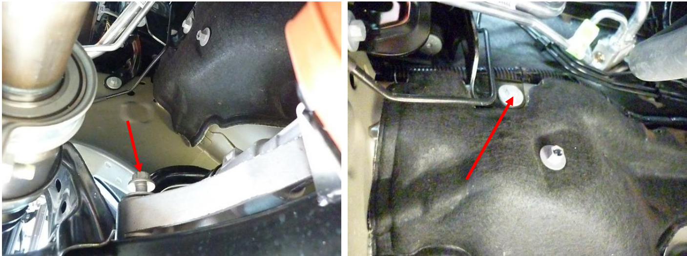
Remove bolts for bracket installation.
