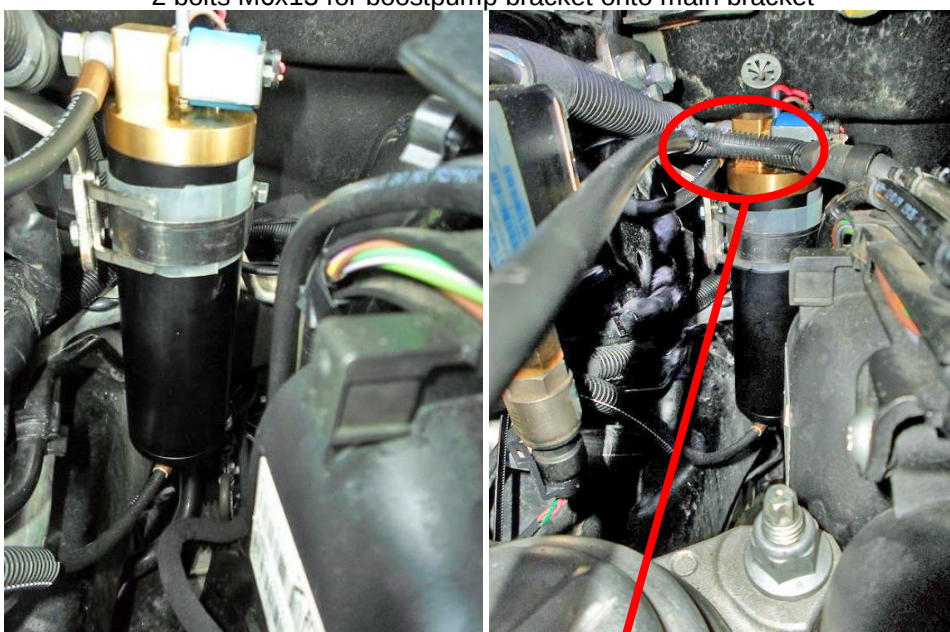
Split-tube Ø9mm protection petrol fuel line
