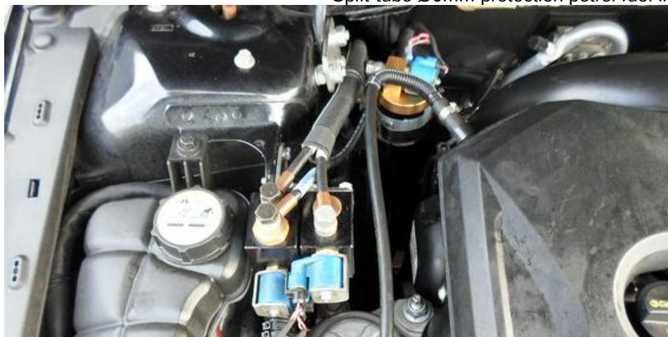
Split-tube Ø9mm protection petrol fuel line
