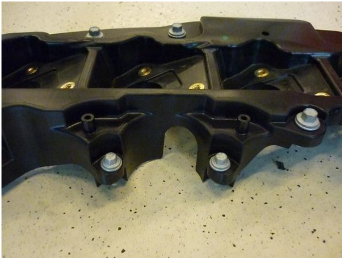
Adapt cover. Remove bolt ( cut away )
