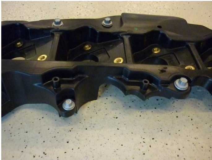
Adapt cover. Remove bolt ( cut away )
