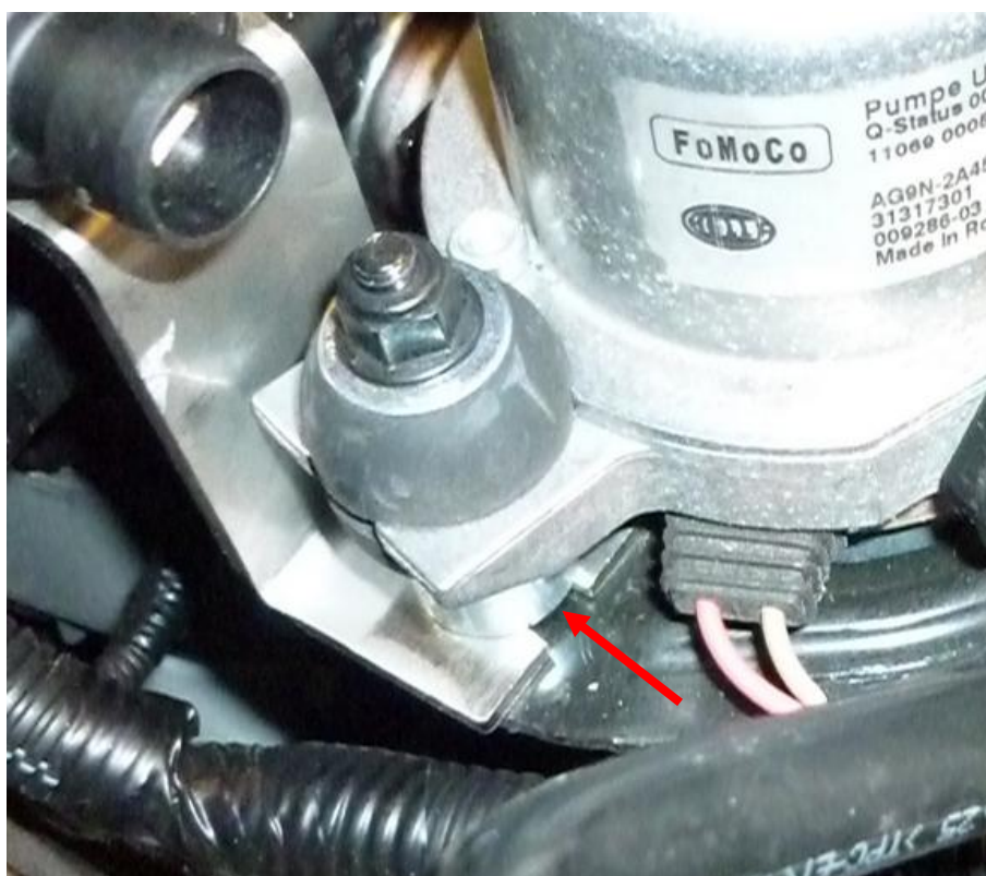
Bracket underneath pump spacer.
