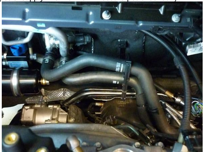
petrol supply hose under coolant hose connections
