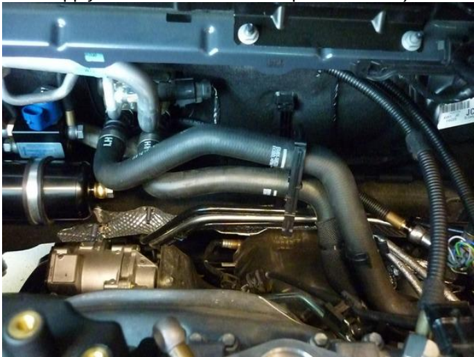
petrol supply hose under coolant hose connections
