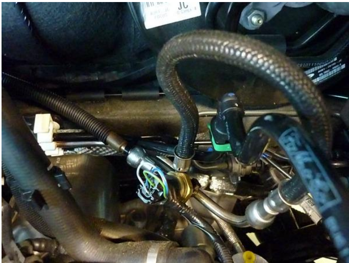
Original hose connected to the boost pump inlet ( petrol supply line with Low Pressure petrol sensor )
