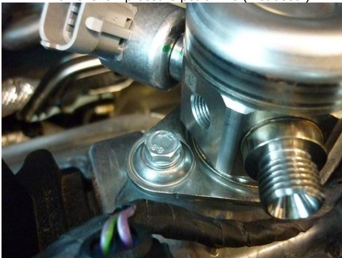
Remove low pressure petrol line ( not used )
