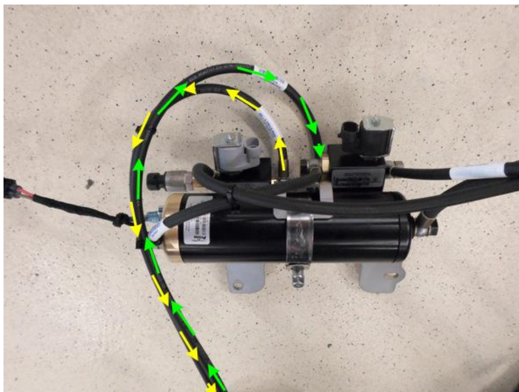
Fuel line and return line to LPG tank.
