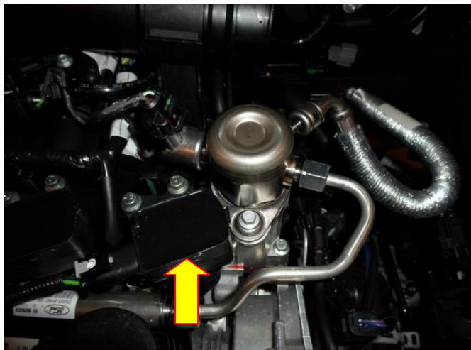
Remove the ignition coil 3th cylinder.
