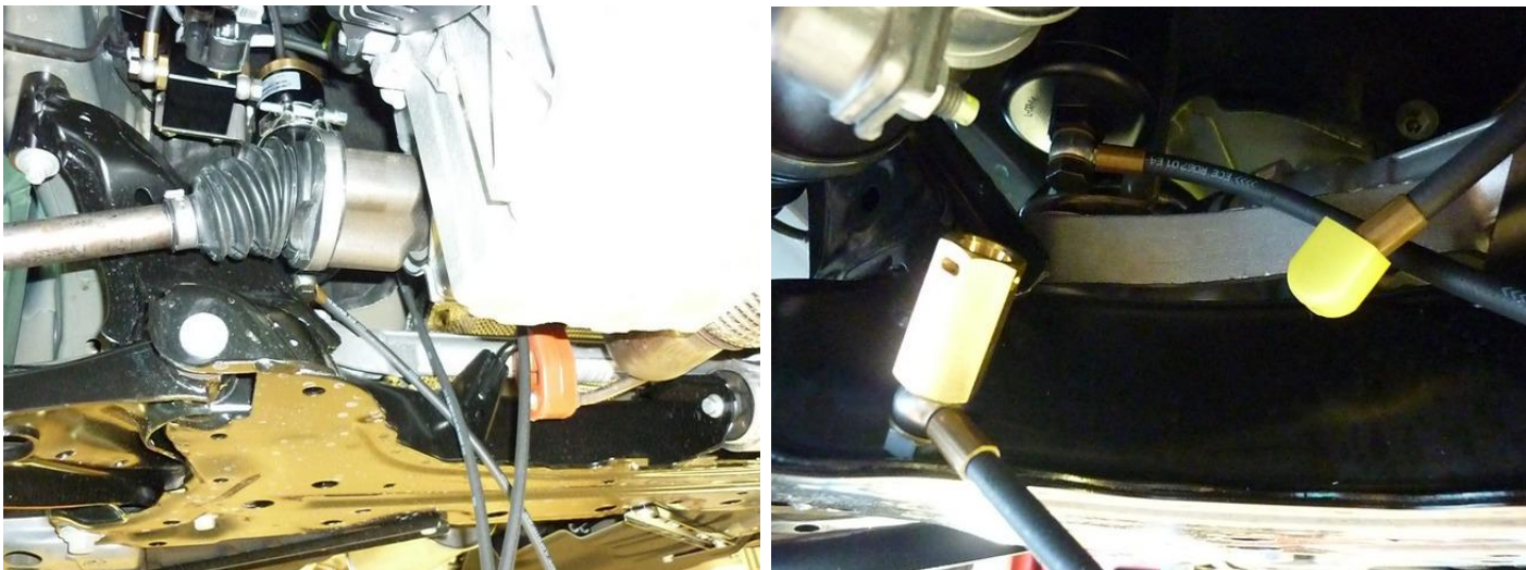
Installed quick connection from boost pump to petrol fuel pipe.
