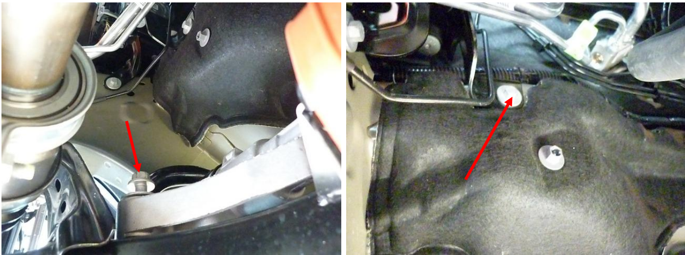
Remove bolts for bracket installation.
