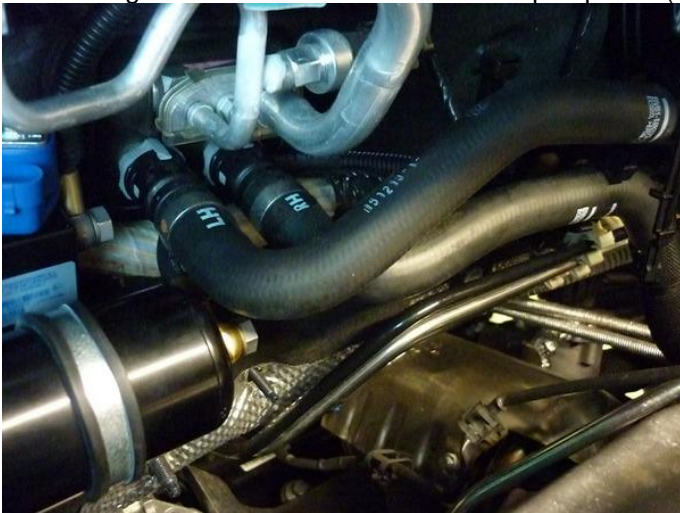
Inlet of banjo eye facing firewall
