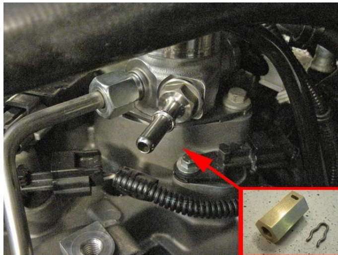
Mount adapter to HP pump. Mount hoses to HP pump.
