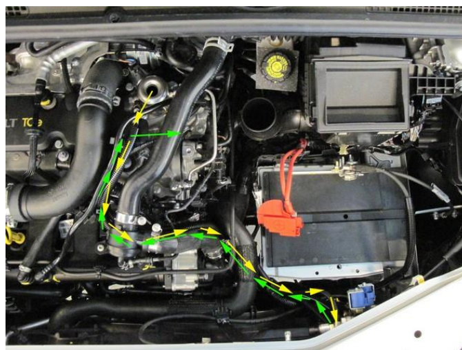
Mount hoses from FSU / FRU to HP pump.
