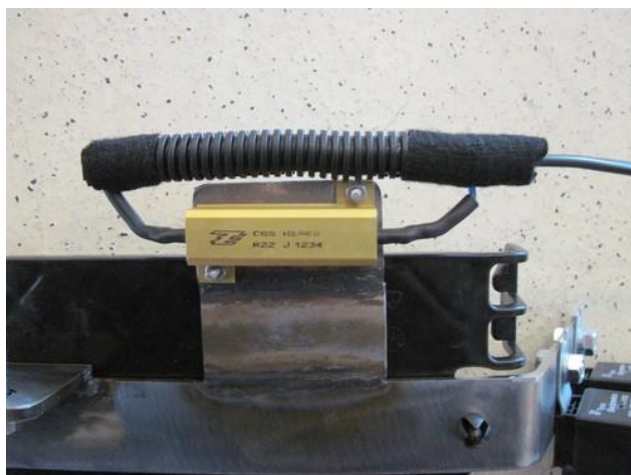
Solder 2-core wire to resistor and use heat shrinks See page 30.
