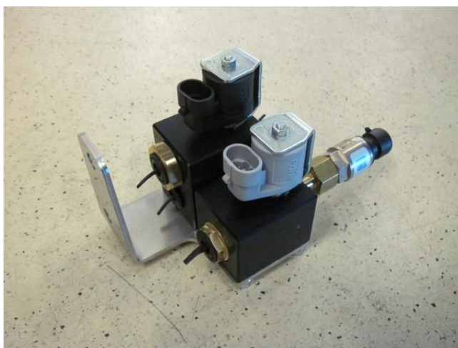
Drill holes Ø9mm and treat anti-rust. Mount FSU & FRU on bracket.
