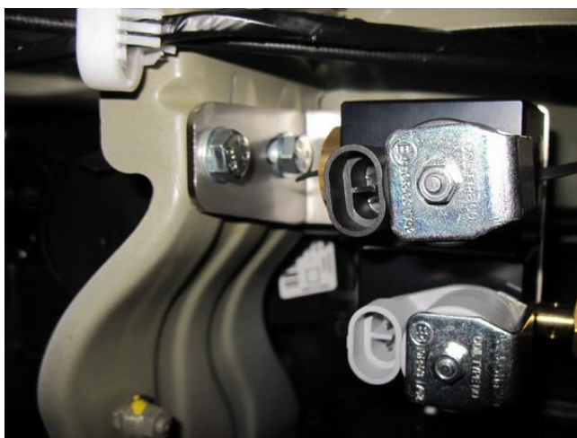
Mount bracket with FSU & FRU to vehicle.
