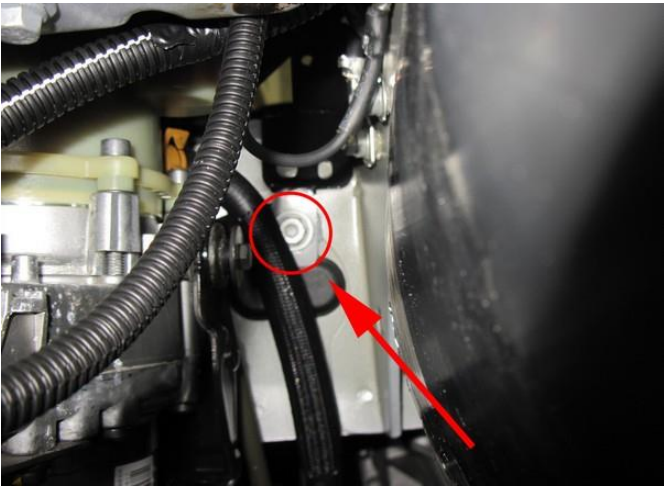
Mount bracket to original bolt from chassis beam next to battery.
