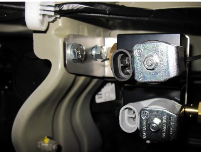
Mount bracket with FSU & FRU to vehicle.
