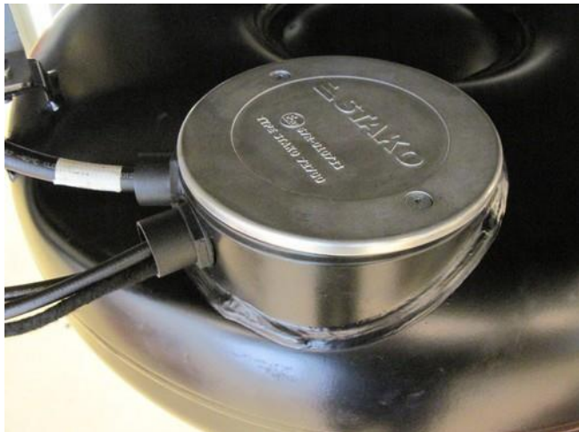
Before tank mounting, mount hoses to tank.
