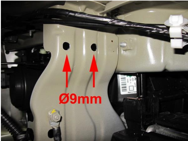
Drill holes Ø9mm and treat anti-rust. Mount FSU & FRU on bracket.
