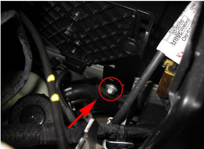
Mount bracket to original bolt from chassis beam. Mount the AFC with dummy connector to the plastic AFC clip
