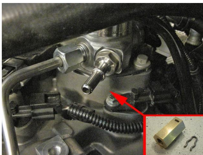
Mount adapter to HP pump. Mount hoses to HP pump.
