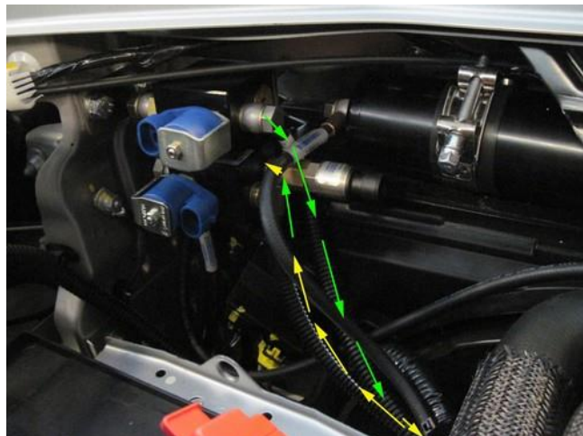
Mount hose from boost pump to FSU. Mount hoses from FSU / FRU to HP pump. Pictures from generation 1 Boost pump, FSU& FRU.
