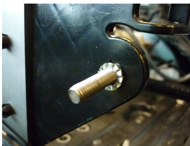
Bolt with (spring or jagged) washer.
