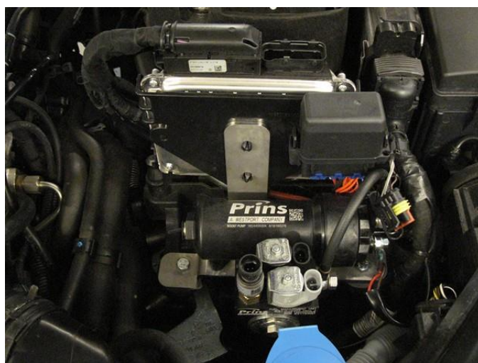
With AFC clip mounted onto bracket.
