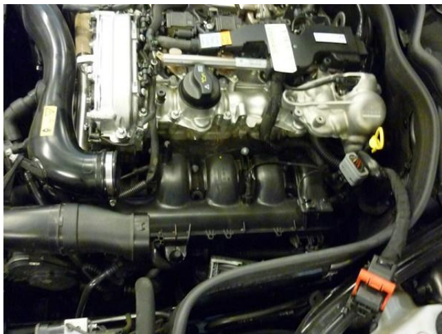
Remove air box with petrol ecu
