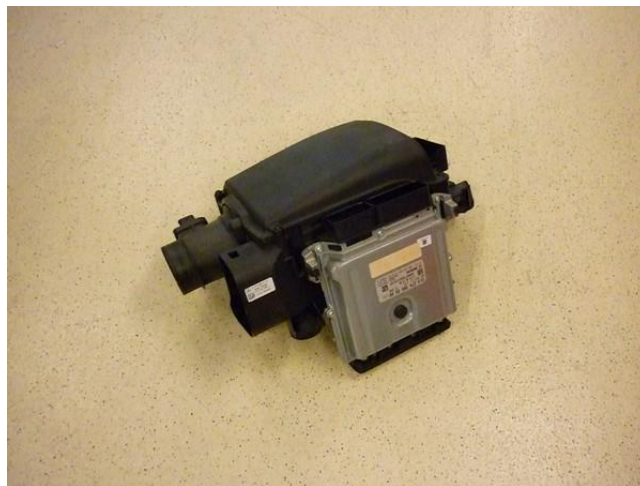
Remove air box with petrol ecu
