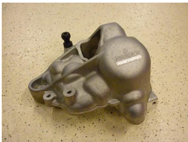
Remove pump cover ( bolts 1-2-3-4 )
