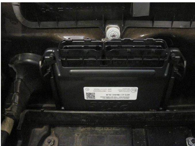
Mount the bracket & mount the AFC.
