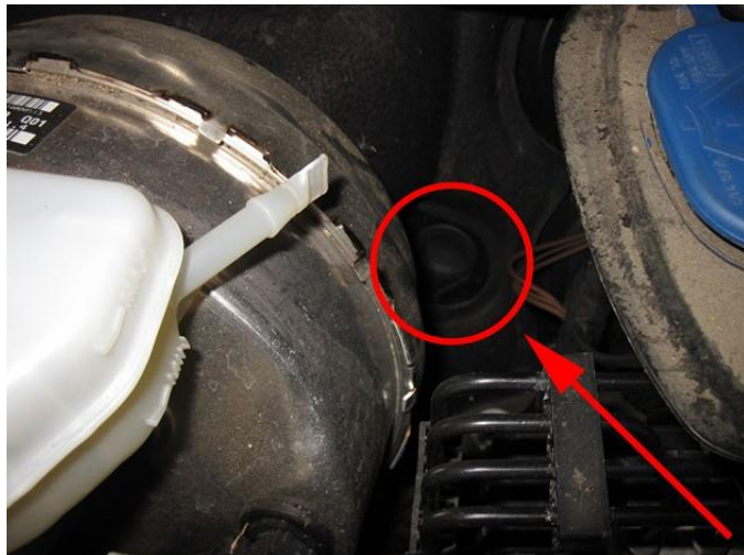
Wiring grommet to the inside of the vehicle.
