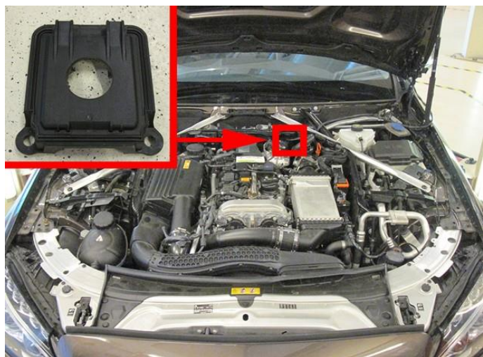
Wiring to the engine room. Drill a hole Ø30mm into the plastic cover/cap for the wire transit.
