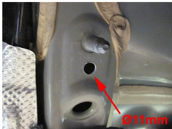
Mark hole and drill Ø11mm.
