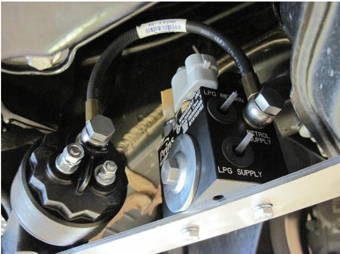
Mount hose between boost pump & FMU.
