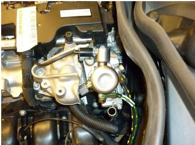
Mount hoses from FMU to the high pressure pump.
