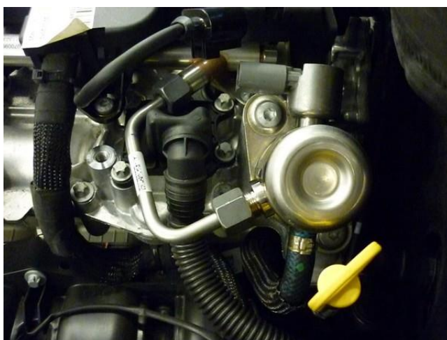
Remove HPP fuel line / fuel hose (and clamp)
