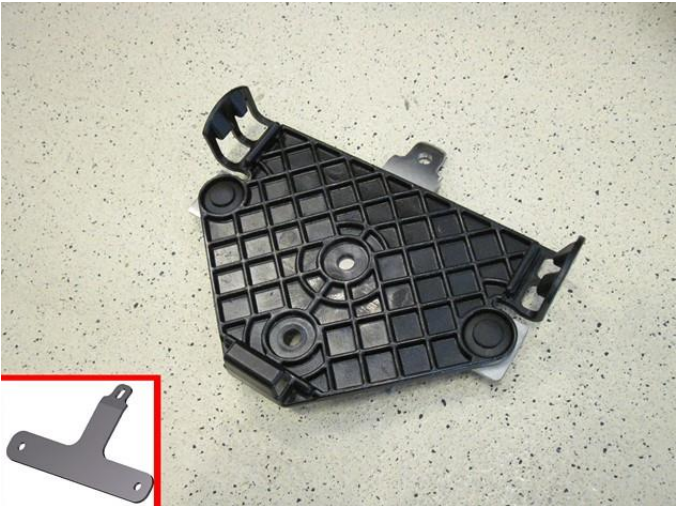
Mount the plastic AFC-clip to the bracket
