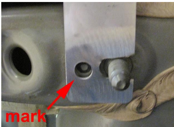
Mark hole and drill Ø11mm.
