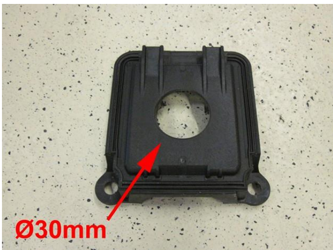
Wiring to the engine room. Drill a hole Ø30mm into the plastic cover/cap for the wire transit.
