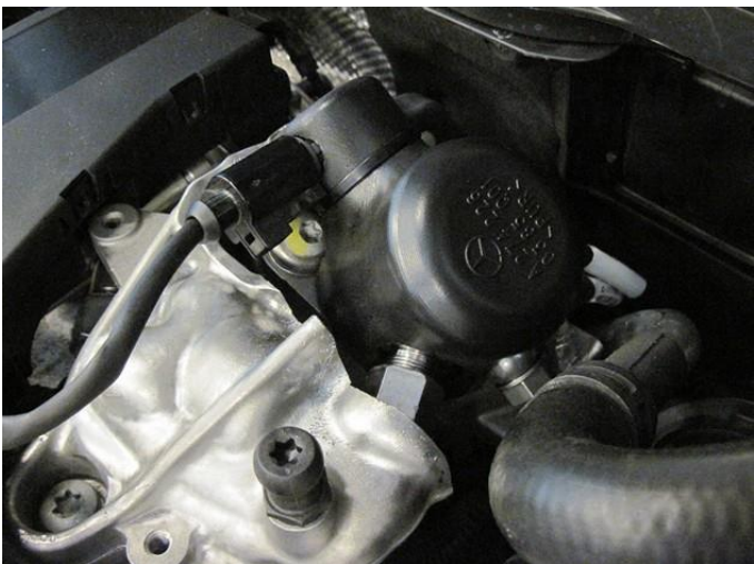
Adapt pump cover and mount to high pressure pump.
