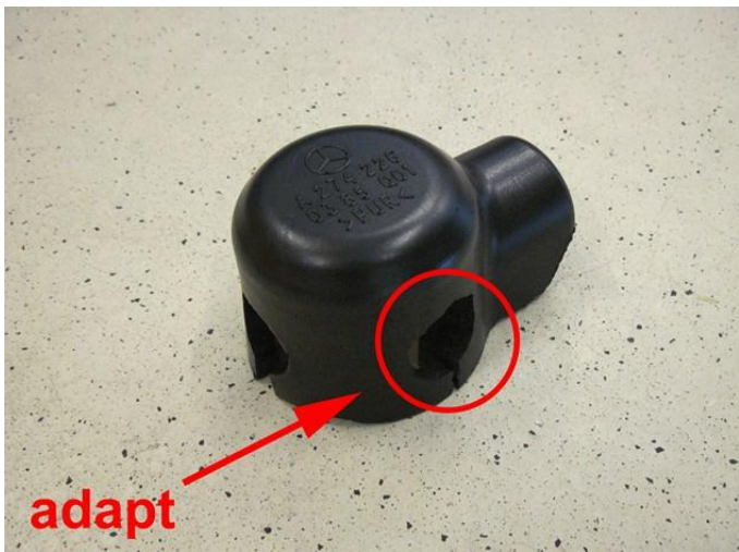
Adapt pump cover and mount to high pressure pump.
