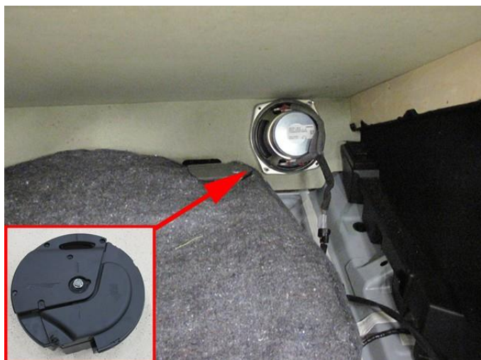
Example: with the option of a subwoofer, remove the speaker from the box and mount to the floor cover. Also drill the hole in the floor cover for the speaker.
