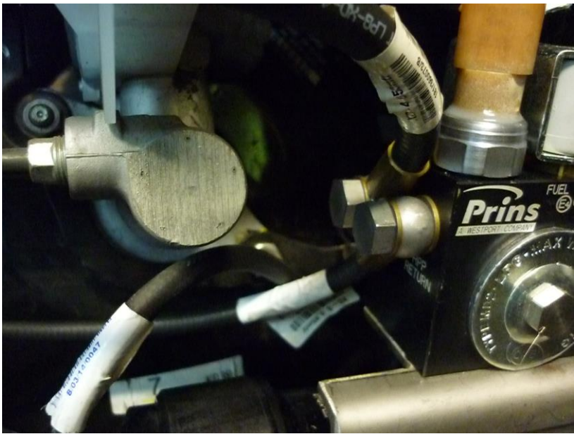
Connect hoses to the boost pump and FMU.
