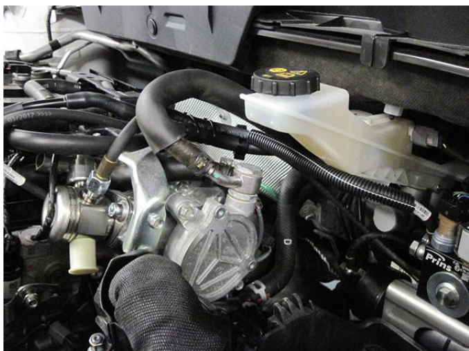
Routing hoses. Mount the extension cable.
