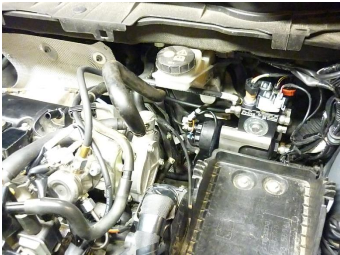
Connect hoses to the boost pump and FMU.
