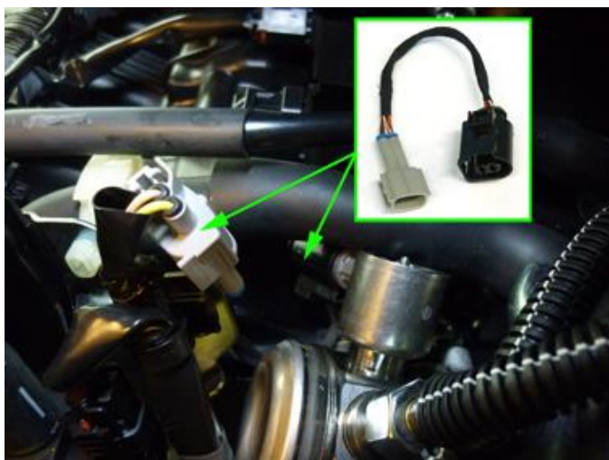
Routing hoses. Mount the extension cable.
