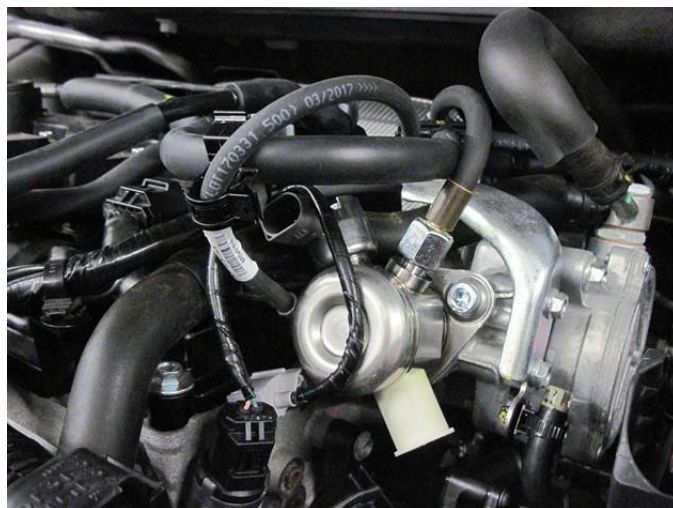
Mount the hoses between the high pressure fuel pump and the FMU.
