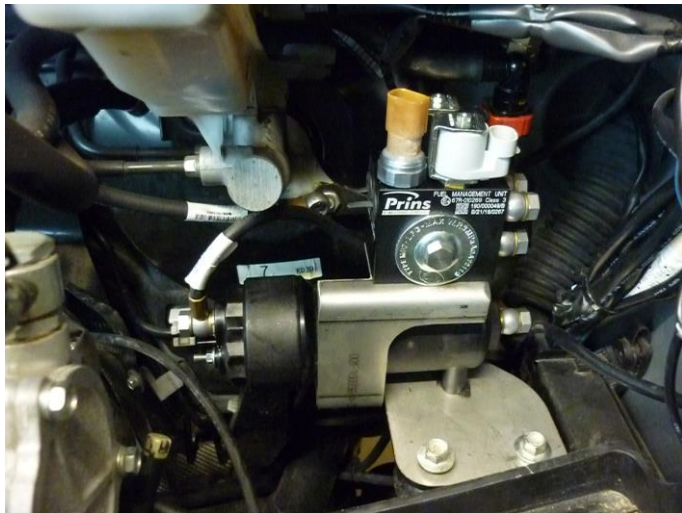
Connect hoses to the boost pump and FMU.
