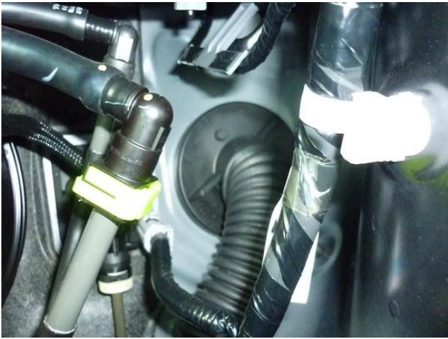
Grommet for transit the Switch,CAN wiring & Fuel reset wires, before installing the fuel unit.
