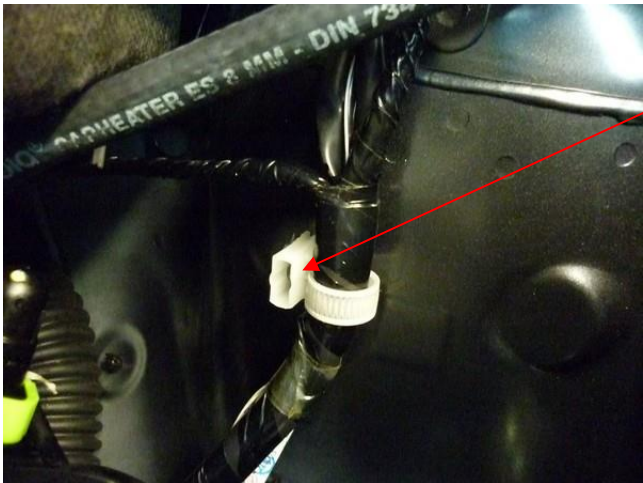
Replace white cable clamp, wiring loom moves to front ( only Mazda 3/6/CX-5 ).
