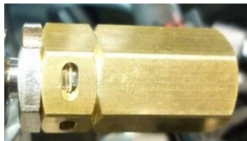
New type quick connector: Tighten with 20Nm.
