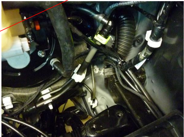
Replace white cable clamp, wiring loom moves to front ( only Mazda 3/6/CX-5 ).
