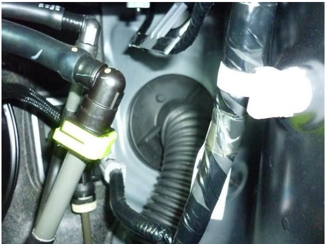
Grommet for transit the Switch and CAN wiring (before installing unit)
