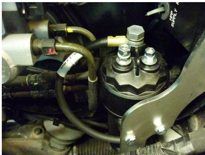
Connect to the boost pump
