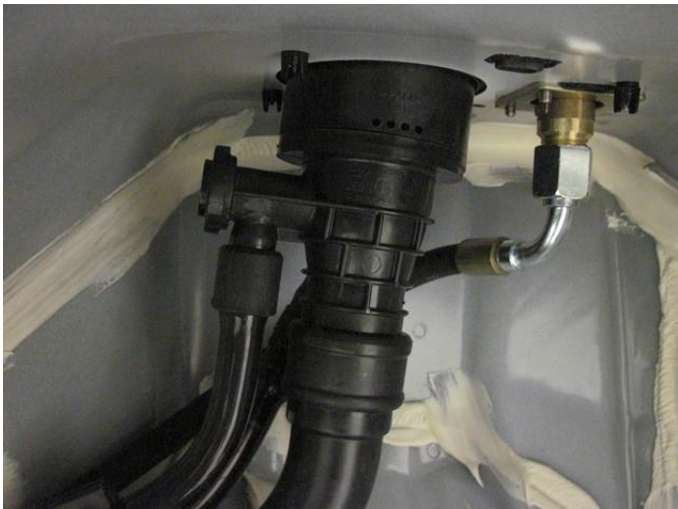
Connect the filler hose to the filler.
