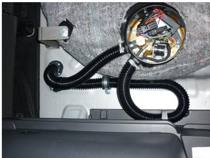
Filler hose ventilation hose, \pm 37 cm Use a 35 mm clamp on supply ventilation hose \pm 85 cm
