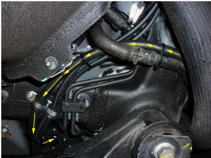
Connect the filler hose to the filler.
