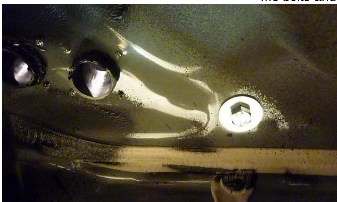
M8 bolts and washer plates
