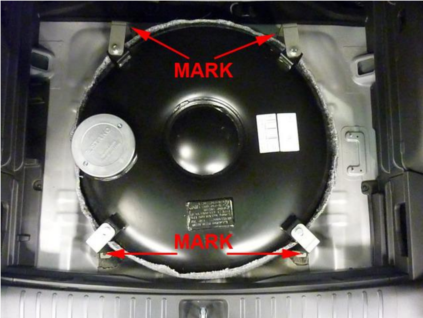
Install tank temporary to mark the holes
