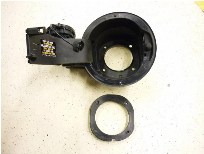
Insert ring before placing bracket
