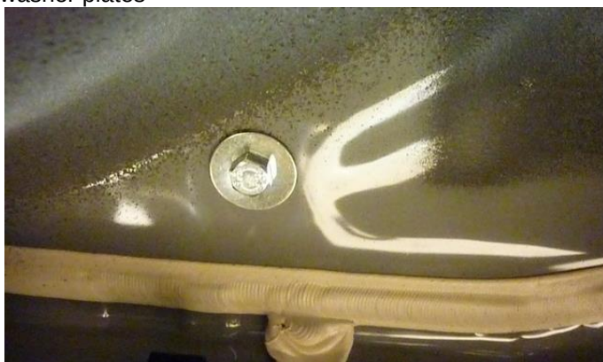
M8 bolts and washer plates
