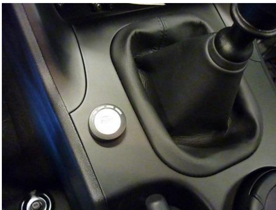
Drill Ø8.3mm, mount the switch
